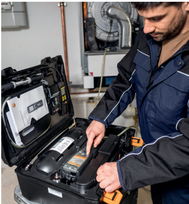
Automatic servicability test with gas-feed appliance with connection to the gas boiler
