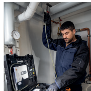
Drinking and waste water test (high-pressure probe up to 25 bar available)
